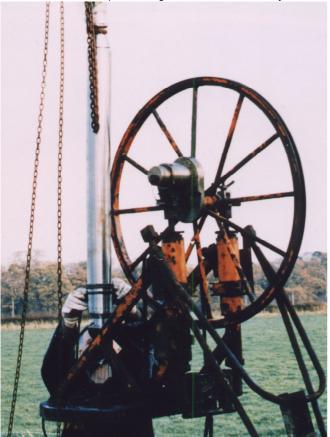
The Mk2 probe is 100mm in diameter and has four rotating highly directional transducers driven by a powerful geared d.c. motor. The Mk2 probe is used to provide cross-sectional profile data of the cavity when the lining tubes have been withdrawn..
